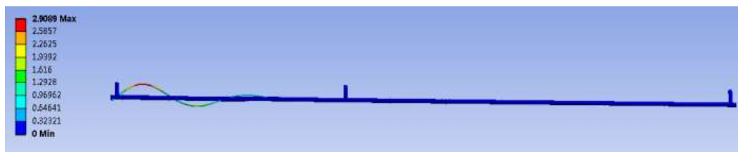
Figure 5. First modal shape of structure
