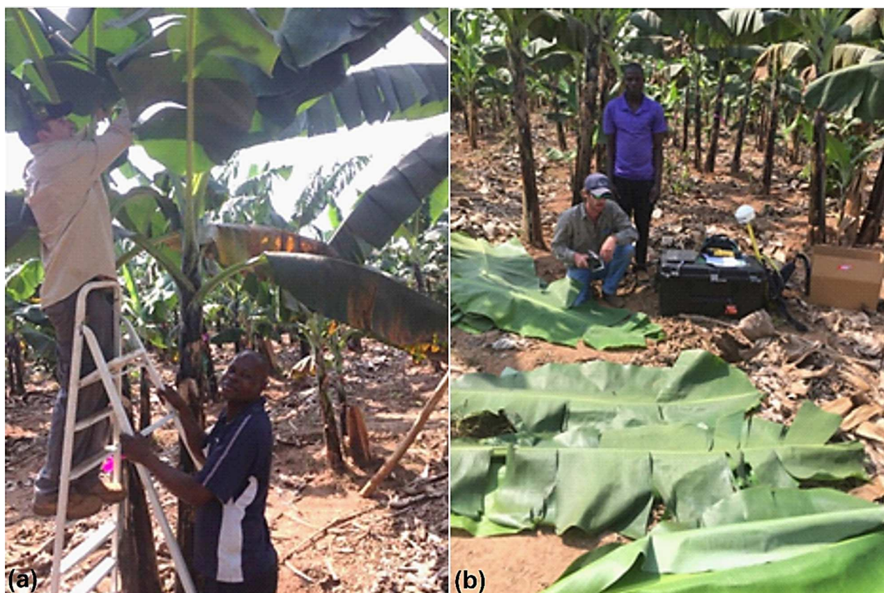
Fig. 2. The manual cutting of sample leaves from each plant (a), followed by the near immediate spectral measure with the ASD field spectrometer fitted with the leaf clip (b).
